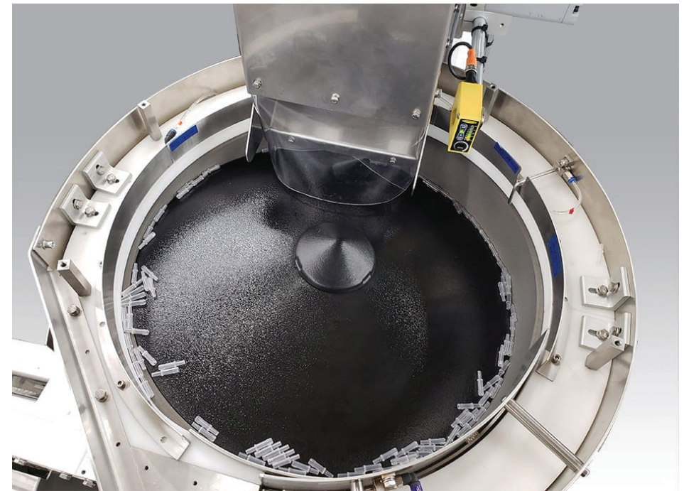
This centrifugal feeder supplies a cylindrical part for a medical device at rate of more than 800 parts per minute. Photo courtesy Performance Feeders Inc.
