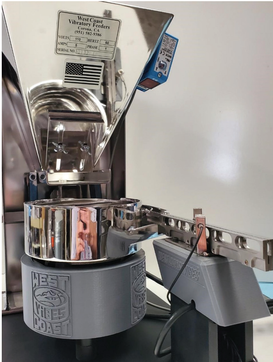
This feeding system delivers a small tungsten shaft for a tool to assemble pacemakers. Photo courtesy West Coast Vibratory Feeders.
