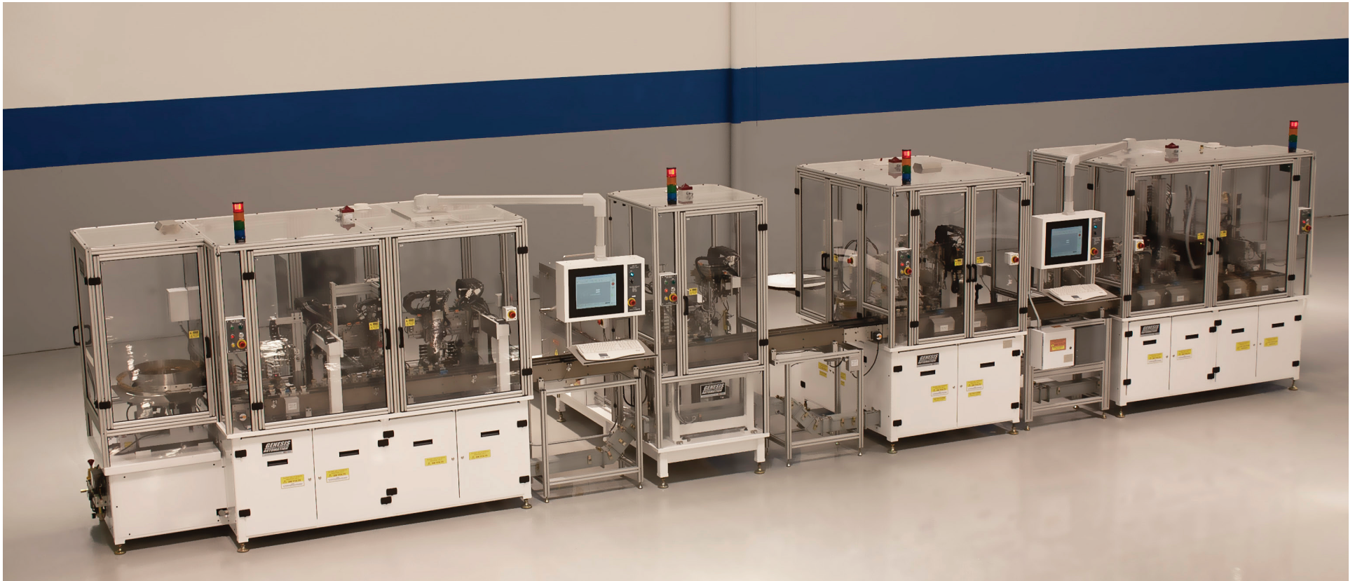
This modular system assembles airflow sensors at a rate of 500 parts per hour. Photo courtesy Genesis Automation.
