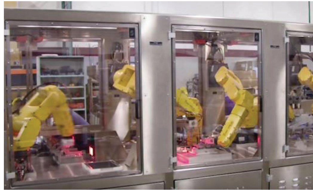
This robotic assembly system can produce 18 syringes per hour. Photo courtesy Farason Corp.
