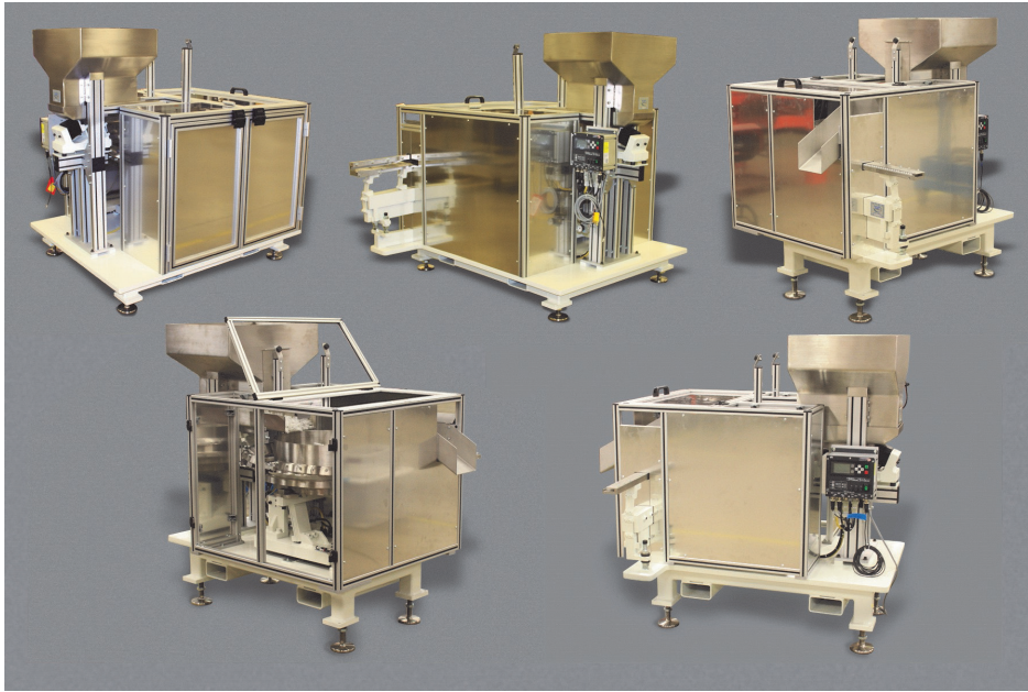
These enclosed feeders supply fluid-collection vials to an automated packaging system. Photo courtesy Fortville Feeders Inc.
