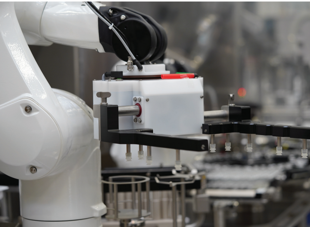
GEH6000IL gripper from Zimmer Group in use at Bausch+Ströbel clean room application
