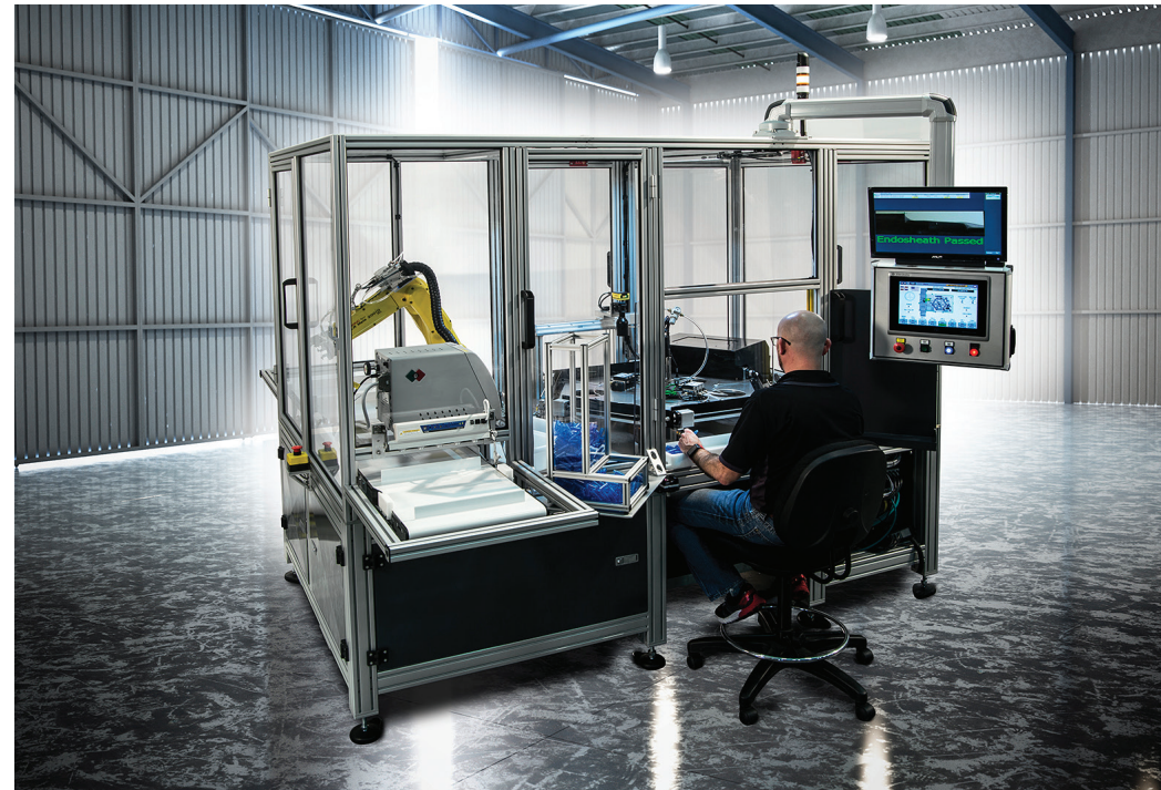
RND Automation designed and built this rotary indexing machine to assemble covers for endoscopic cameras. It assembles approximately four covers per minute. Photo courtesy RND Automation.
