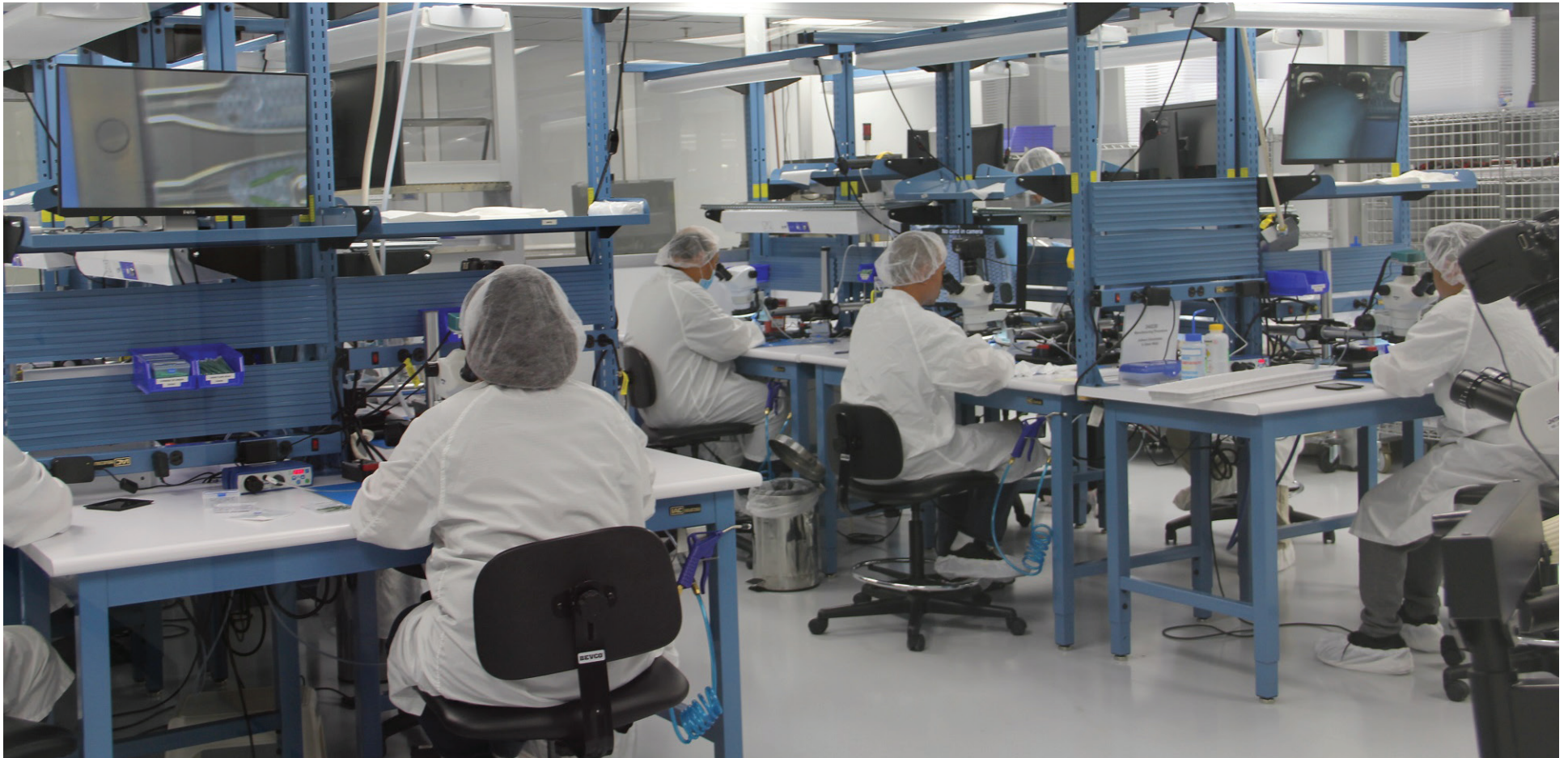
Cirtec's headquarters in Brooklyn Park includes two Class 10,000 clean rooms. Photo courtesy Cirtec Medical Corp.
